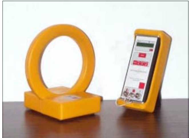
Figure 5. Close-up view of reader and standard benchtop antenna.
