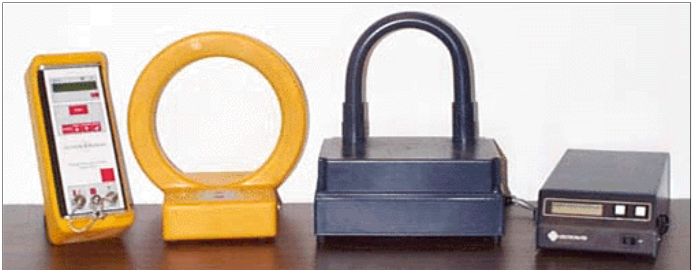
Figure 7. Standard benchtop antenna and portable reader, shown with the 400kHz blue-loop reader and antenna.
