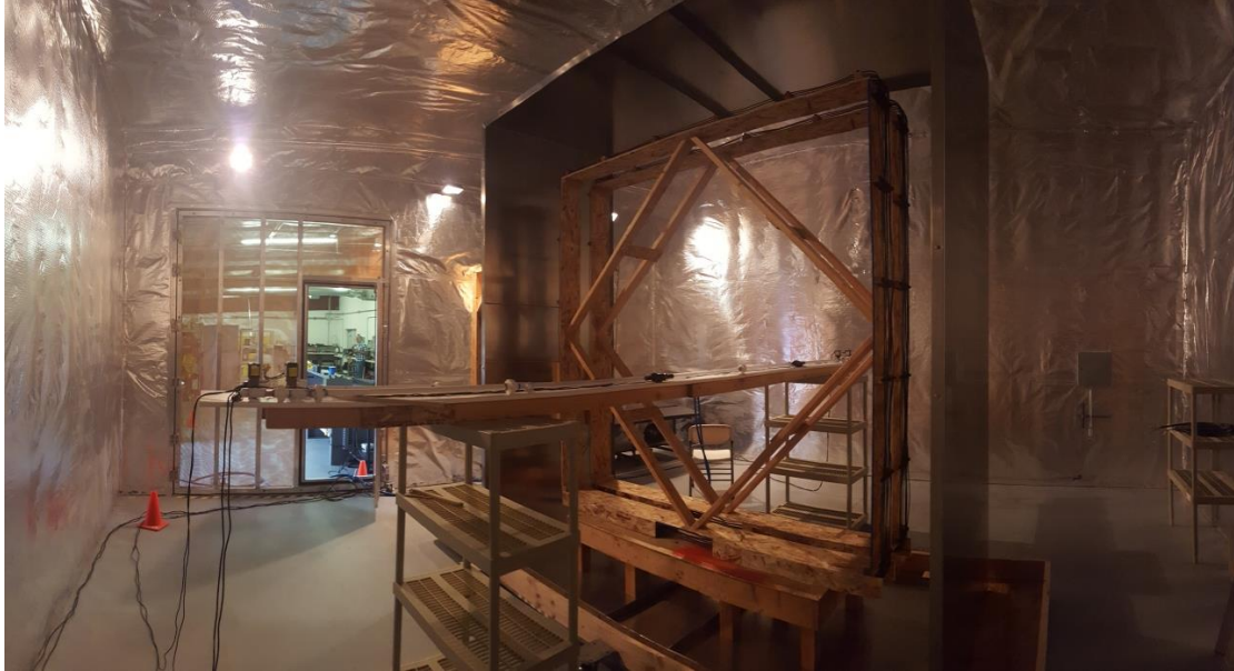
Figure 2. Photo of the \frac{1}{2} -scale model of the BCC antenna. Note the RF shielded room, aluminum shield and pneumatic shuttle.
