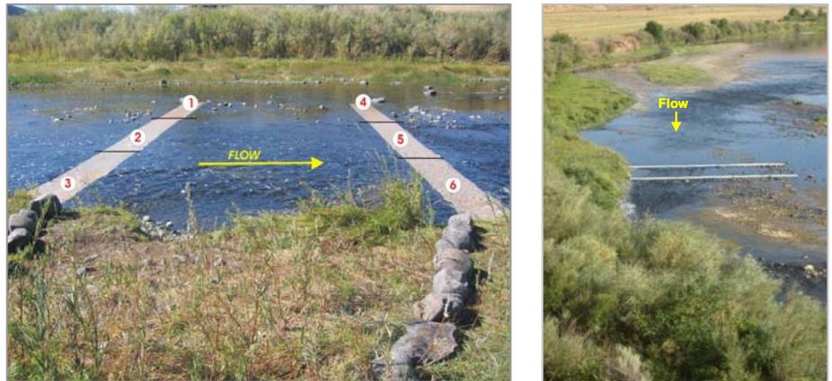
Figure 3. Photos showing the six antennas in the two 3-antenna array configuration
