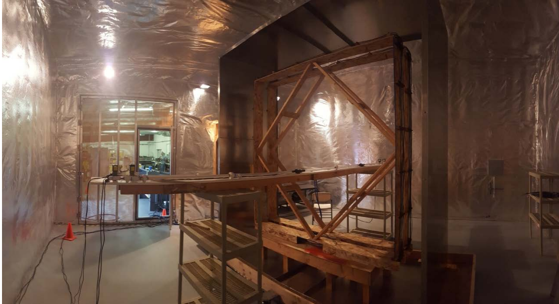
Figure 2. Photo of the 1/2-scale model of the BCC antenna. Note the RF shielded room, aluminum shield and pneumatic shuttle.
