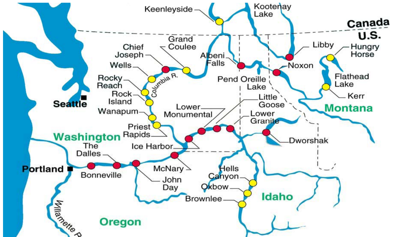
Figure 1 Hydroelectric projects on the Snake and Columbia Rivers. This figure is reprinted courtesy of the U.S. Army Corps of Engineers, Portland District. Red circles are Corps of Engineers projects, yellow circles are privately owned or Bureau of Reclamation projects.
